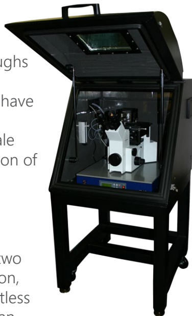
AEK-2002 + TS-150 Supporting An Asylum Research AFM
