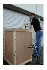
Remove panel labeled 'Front' by removing marked screws.
