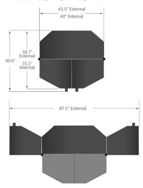
Internal Dimensions (W x D x H): 40 x 35.1 x 38 inches / External Dimensions (W x D x H): 43.5 x 40.6 x 67.5 inches
