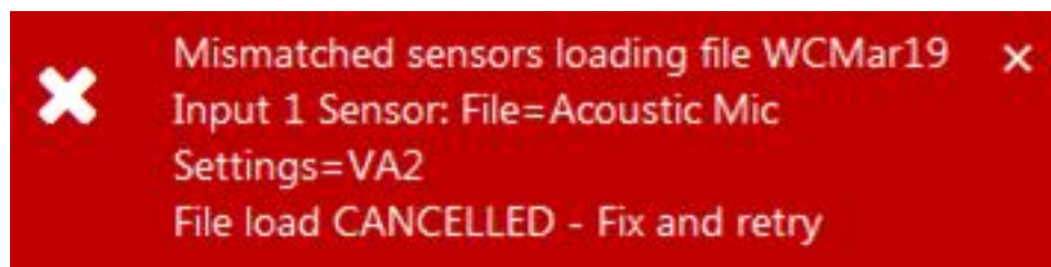
Figure 5: Warning prompt when sensor and input units of the save file do not match the existing measurement plot.
