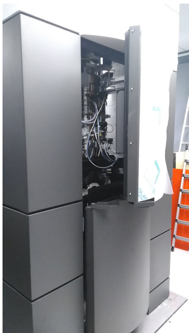
Custom AVI-600 Platform and Support Frame Supporting a FEI Krios TEM and Acoustic Enclosure
