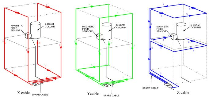
Aluminium frames to carry the cables are available from Spicer Consulting. The joints are insulated to ensure that there are no shorted loops in parallel with the cables. Similar precautions must be taken if the frame is obtained locally, otherwise the cancelling performance will be compromised.
