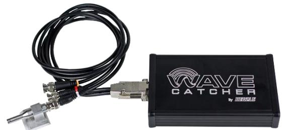
**Figure 2:** Acoustic Microphone Connected to WaveCatcher ADC
