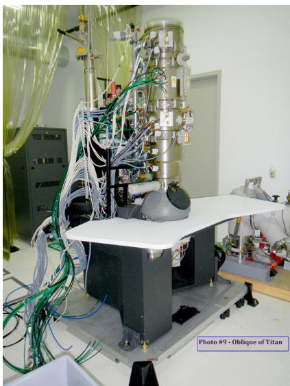
Custom AVI-600 Platform and Support Frame Supporting a FEI Krios TEM and Acoustic Enclosure
