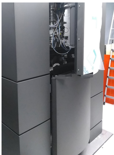
Custom AVI-600 Platform and Support Frame Supporting a FEI Krios TEM and Acoustic Enclosure
