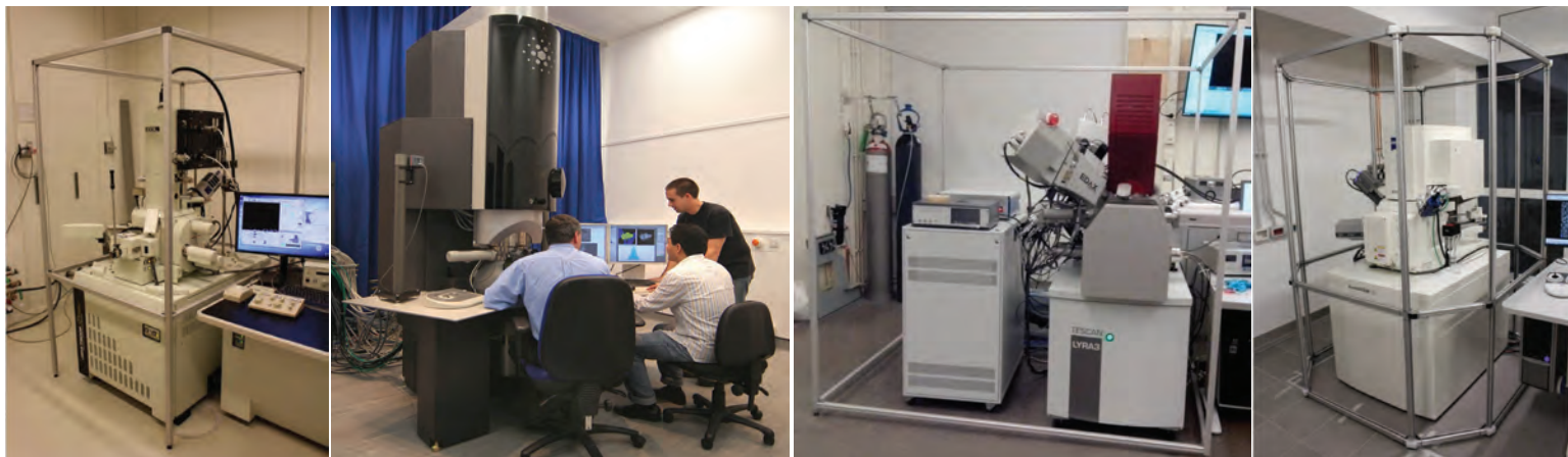
AC and DC Magnetic Field Cancellation for All Electron Microscopes | Integrated Into the Profile of the Room or In A Surrounding Frame
