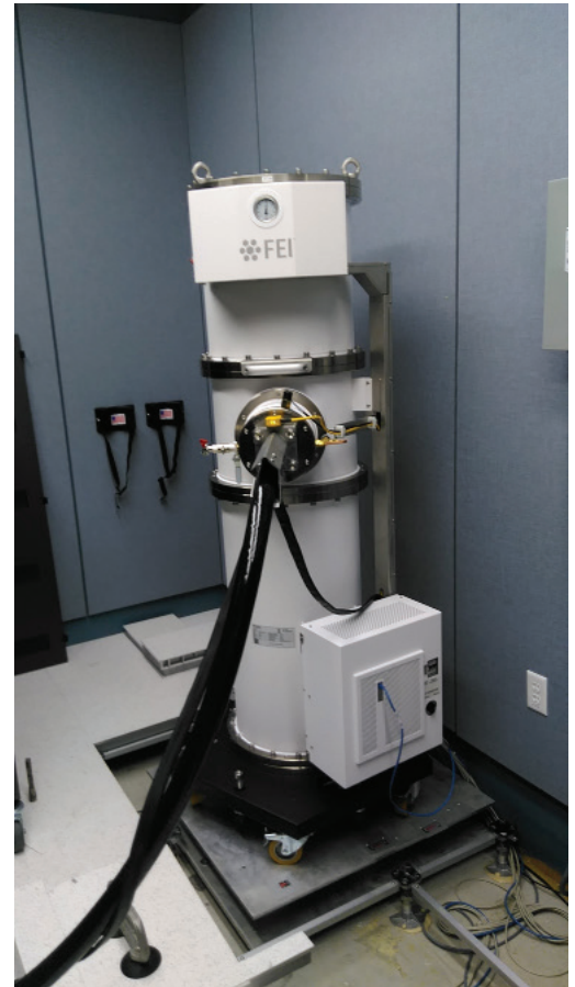
AVI Platform and Support Frame Supporting A TEM's HT Tank In A Lab with A Raised Floor
